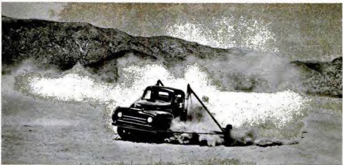
Test truck makes hundreds of wrenching turns in the figure-eight test. Outrigger prevents it from rolling over
